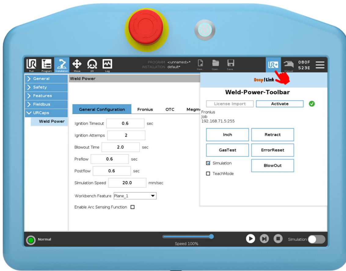
Figure 28 Toolbar presentation, starting from version 1.0.3-Build026, a spot welding button has been added in Toolbar panel, the job number is fixed at 22 for all power source brands.
