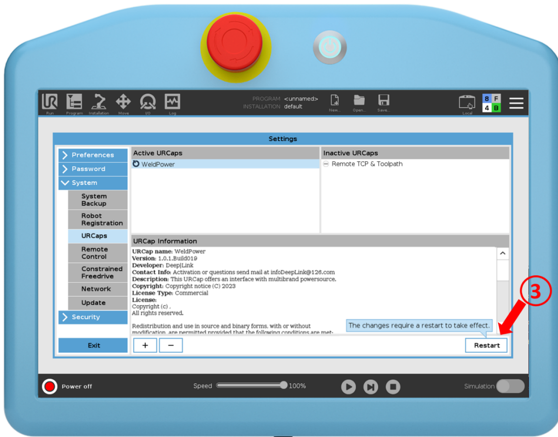
Figure 3 Installation 3rd step
