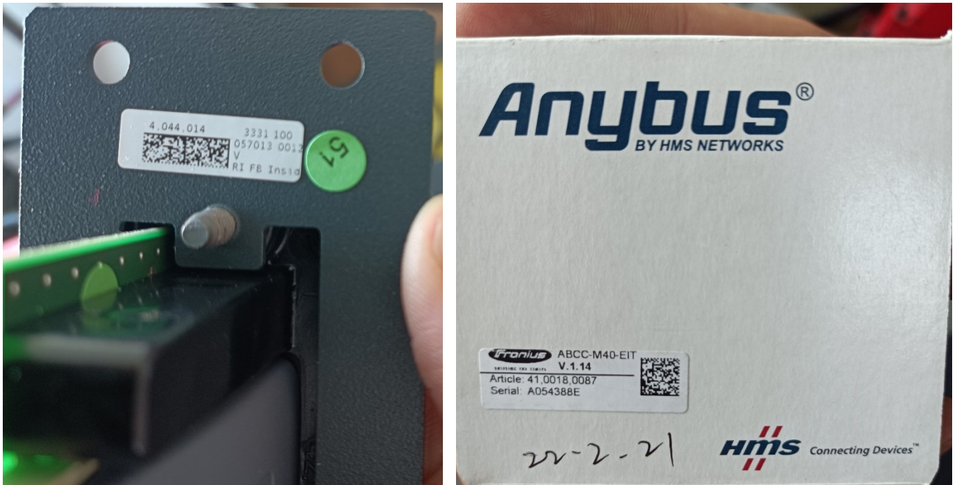
Figure 13 Fronius communication hardware: 4.044.014 of FB module and 41.0018.0087 of Modbus module.
