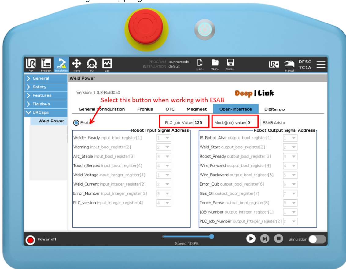
Figure 22 ESAB powersource configuration interface, default ESAB IP address 192.168.0.3, mode 0 (Job).
