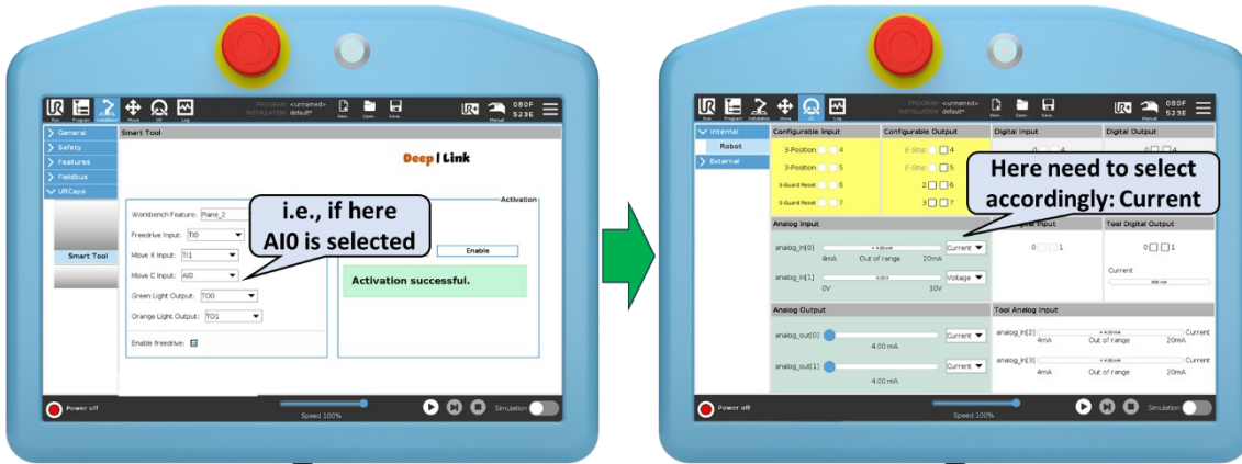
Figure 7 UR20/UR30/UR15/UR18/UR8L cobot IO setting procedure.
