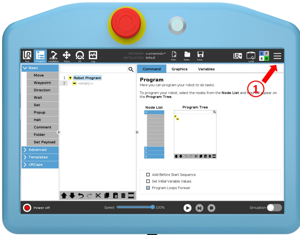
Figure 1 Installation 1st step.
